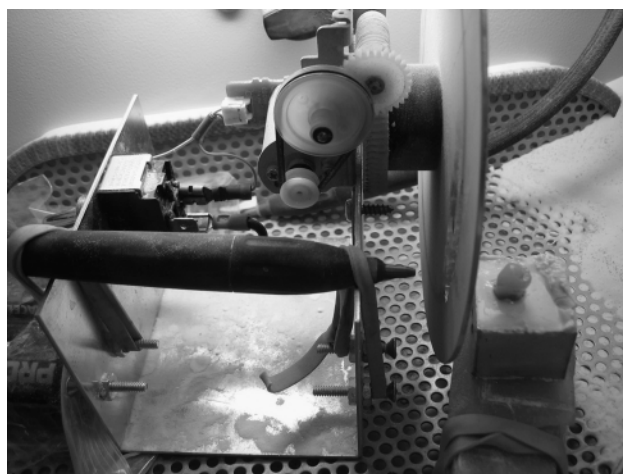
Figure 1 Mounted tooth undergoing air abrasion treatment through the aperture of rotating wheel.
